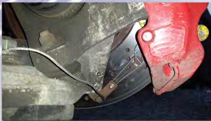
Above, rubbing thermocouple installation
